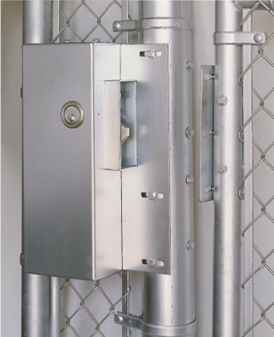
8055 gate lock shown in closed and deadlocked position. When the gate is closed, the locking bolt is completely concealed.
